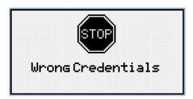
**Note:** In case that invalid UserID or PIN are entered, the controller shows Wrong Credentials screen. Use Enter button to enter Login again or Page Button to go back to menu.
