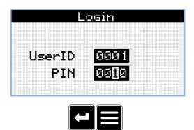
Note: Use Enter button to confirm the PIN and Loging or Page button to cancel entering the Login.
